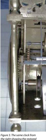
Figure 3. The same clock from the right showing the restored balance wheel escapement. Limited decoration to the hammer stop. Strike fly in line with the wheelwork. Photograph courtesy of Jack and Ann Mcbroom.
