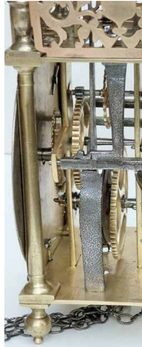
Figure 3. The Lothbury movement of the Civil War period has some interesting early features, such as strongly-tapered arbors to the original wheelwork.
