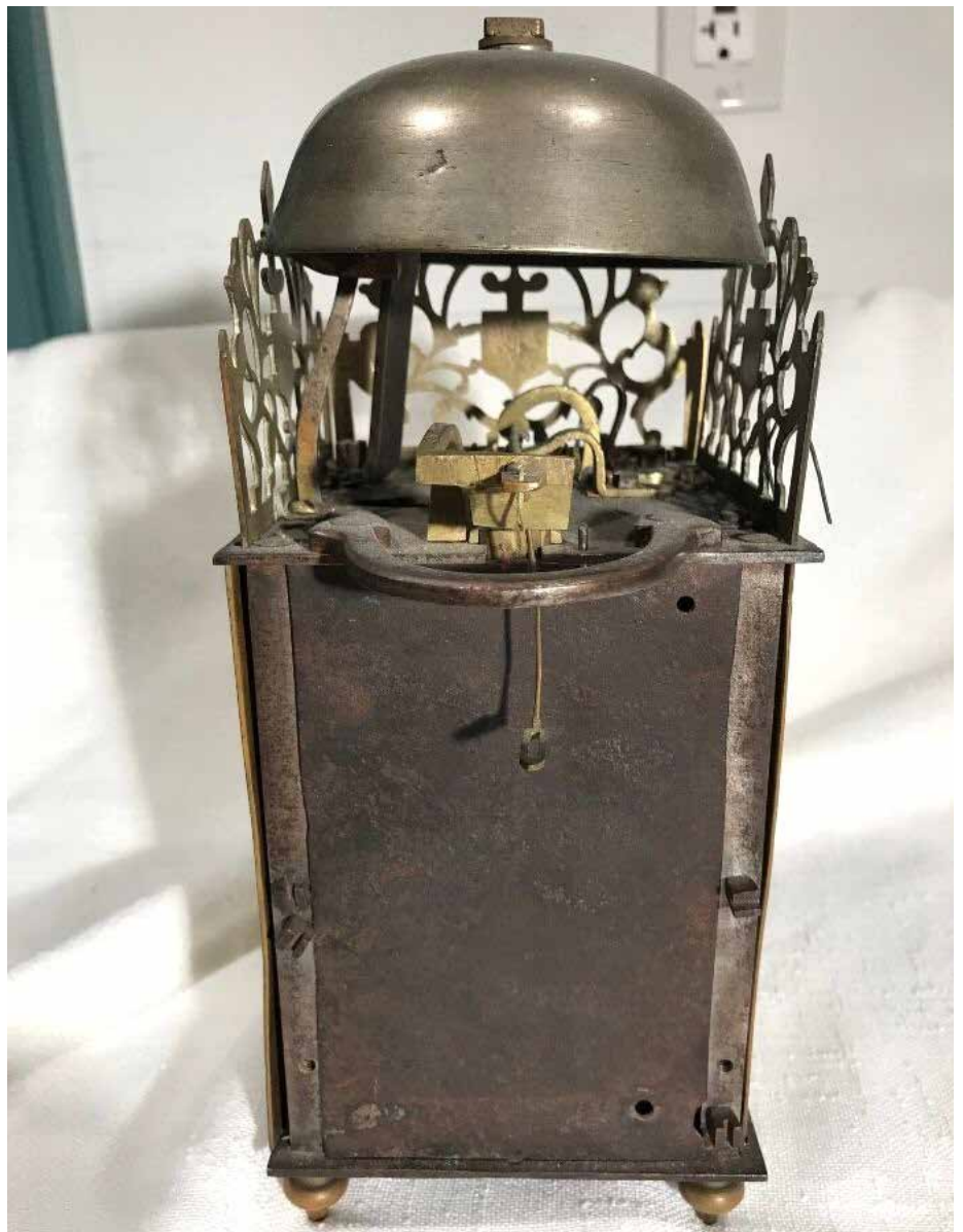
Figure 5. This back view shows he used an exceptional amount of iron, probably to keep the price down. Photograph by Thomas Meyer.
