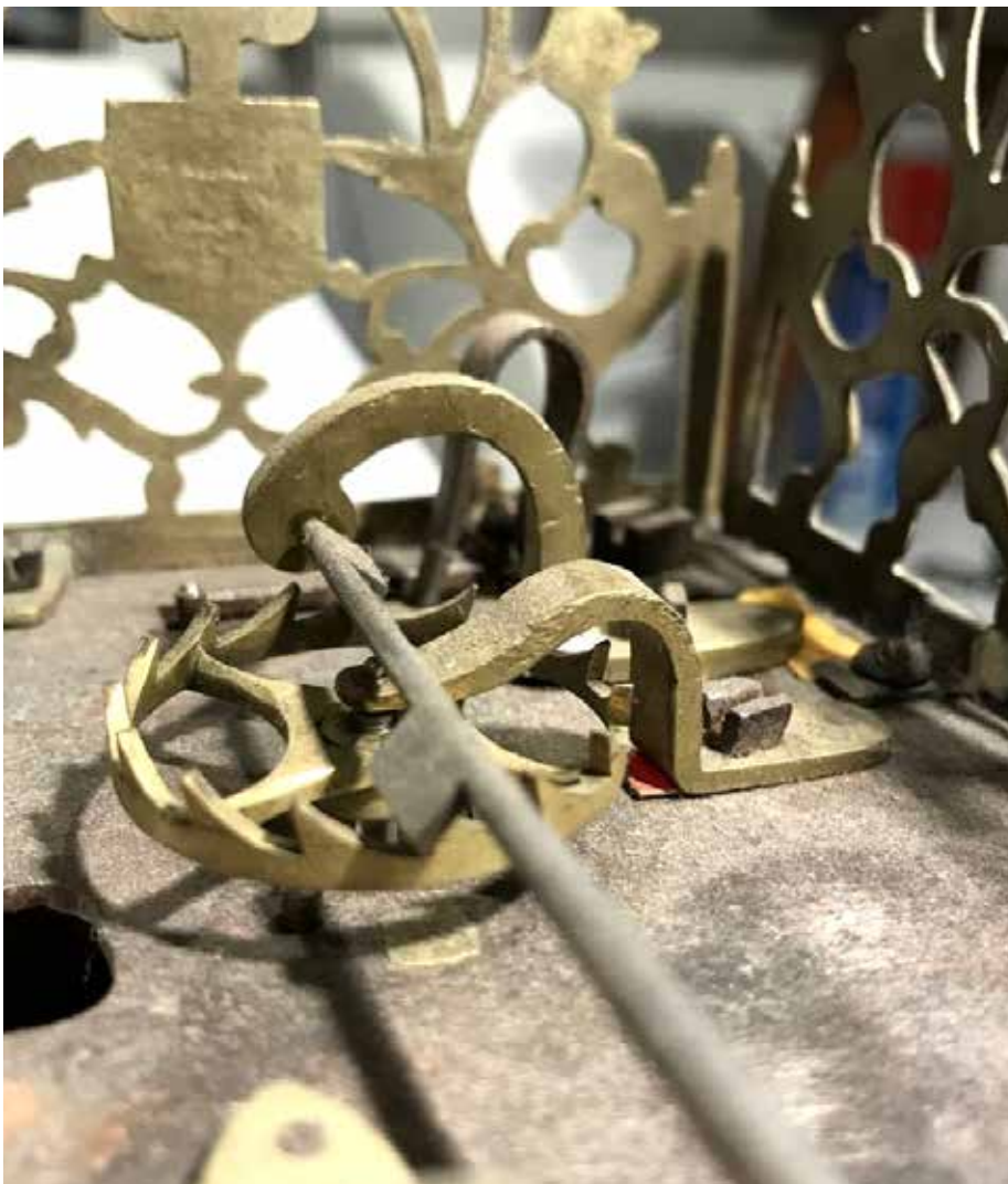
Figure 3. The verge escapement has curved support cocks, typical of French work. Photograph by Thomas Meyer.
