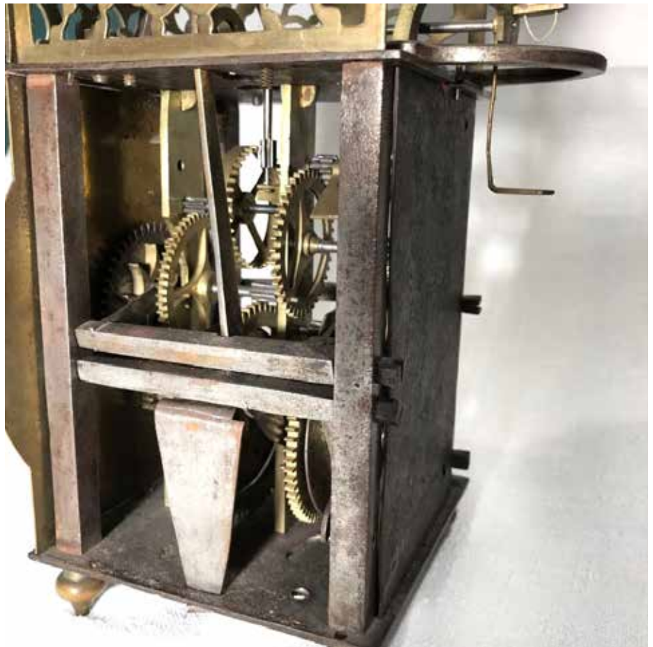
Figure 4. The Guery movement from the right showing the verge escapement set-up. Photograph by Thomas Meyer.
