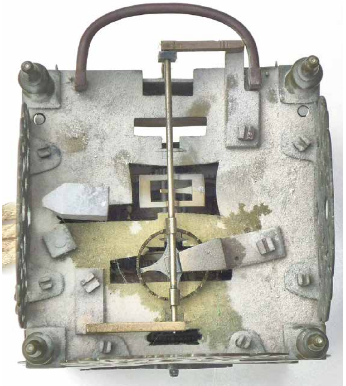
Figure 4. Top plate of the lantern clock. Two vacant holes show where the verge cock was attached before it was re-positioned, probably during some past restoration.
