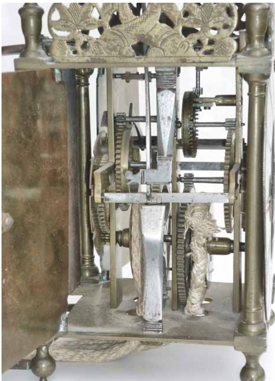
Figure 2. This left view of the lantern clock shows the original verge escapement and the decorative filing to the hammer spring and hammer stop. Pictured before cleaning.
