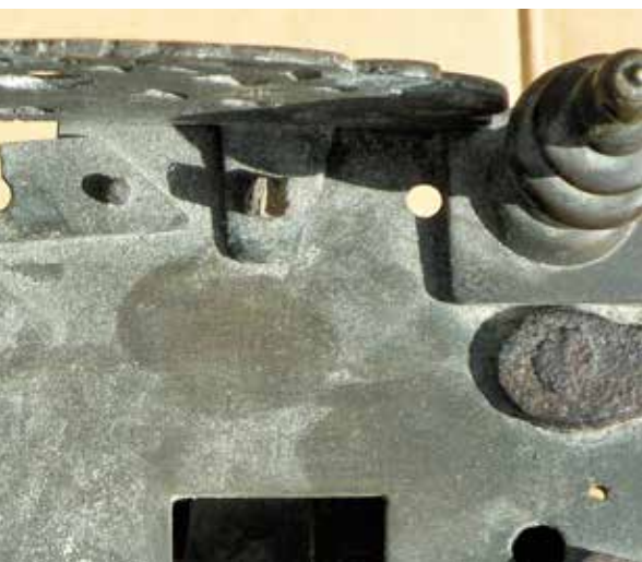
Figure 7 (middle). This view from under the clock shows the normal dial lug hole in the base plate and the fact that the top plate was never drilled for the normal dial top retaining pins.
