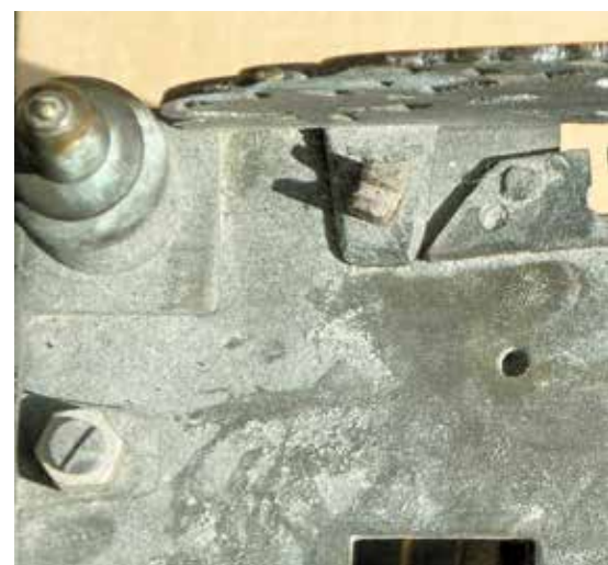
Figure 6 (top). The clip behind the fret fits down between chapter ring and dial plate to hold the dial in place. John Dennis's own device, which is probably unique.
