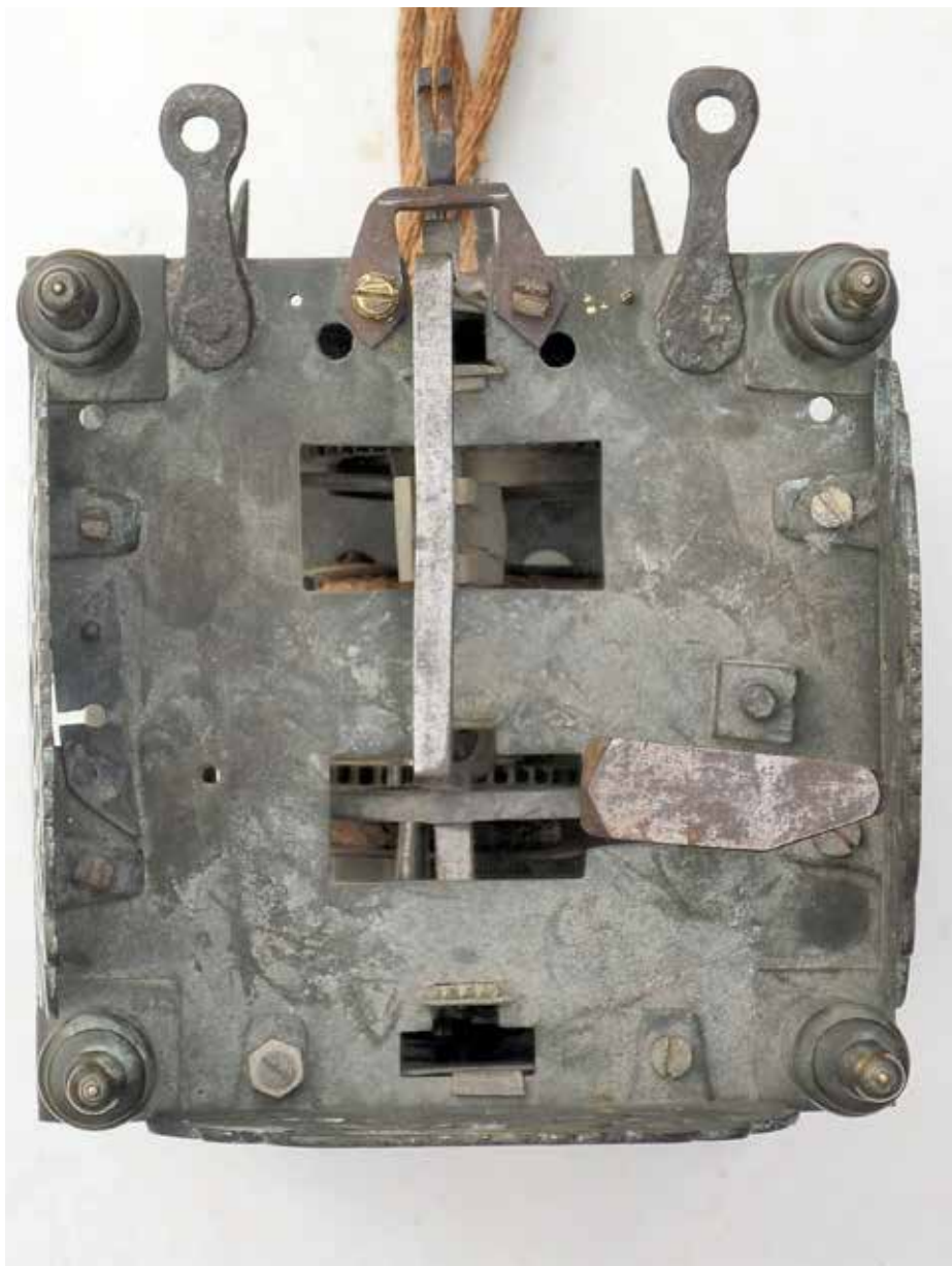
Figure 5. The top plate showing the ancient conversion from balance to anchor. Two empty holes show where the hoop was first attached, moved to make room for the pendulum when converted, and replaced anciently by two individual hoops. A clip behind the front fret and a patch behind the left fret can just be made out.
