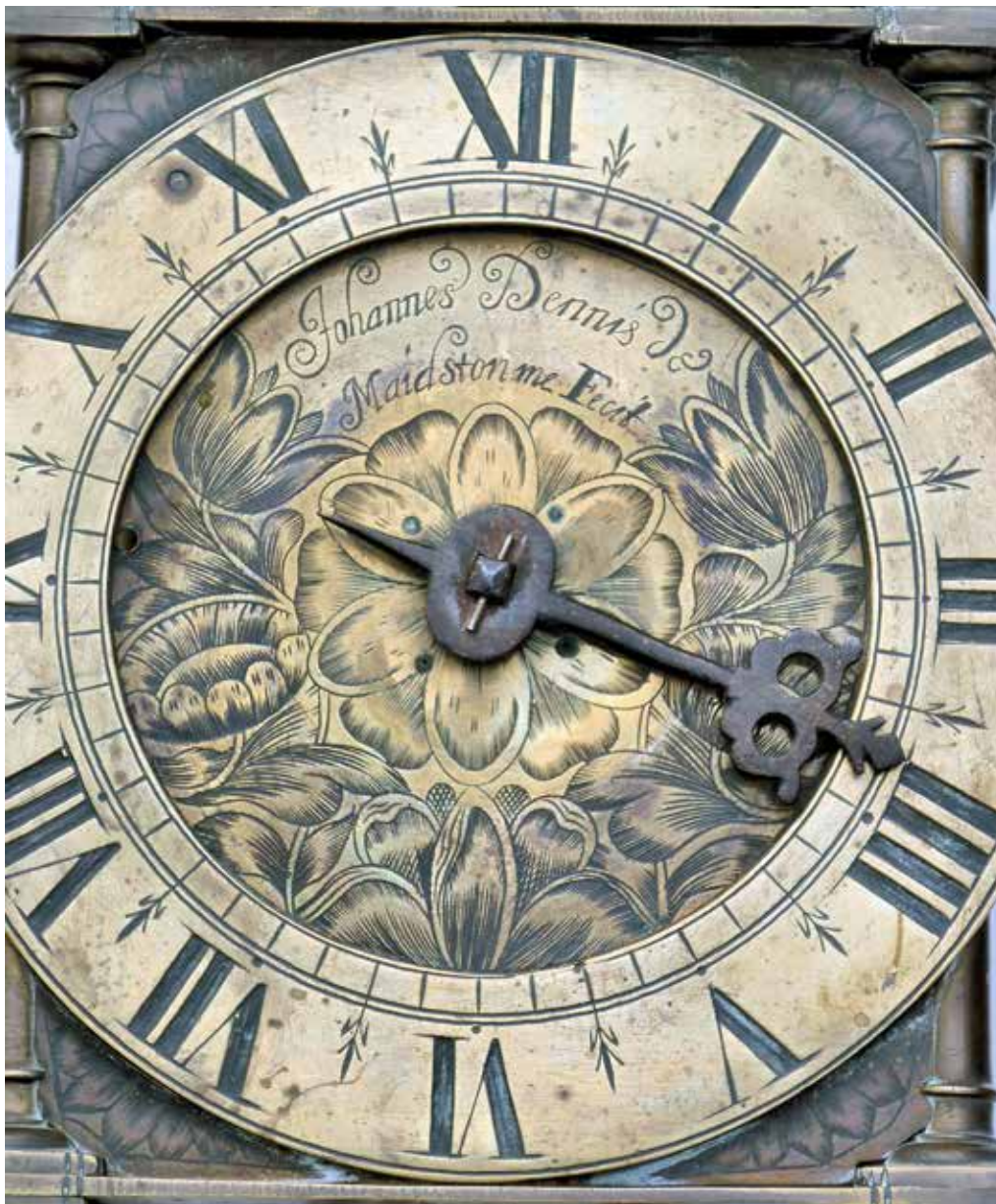
Figure 2. The dial centre detail shows the hole at XI, which carried the original alarm detent. London style engraving and hand. Four holes round the centre are where the alarm disc was once riveted.
