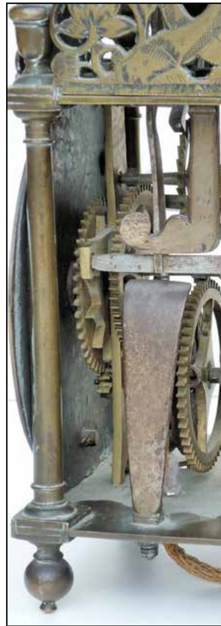
Figure 3. Movement from the right showing the decorated hammer stop. Note the tapered arbors, including that of the escape wheel—an early feature, usually pre-1700.
