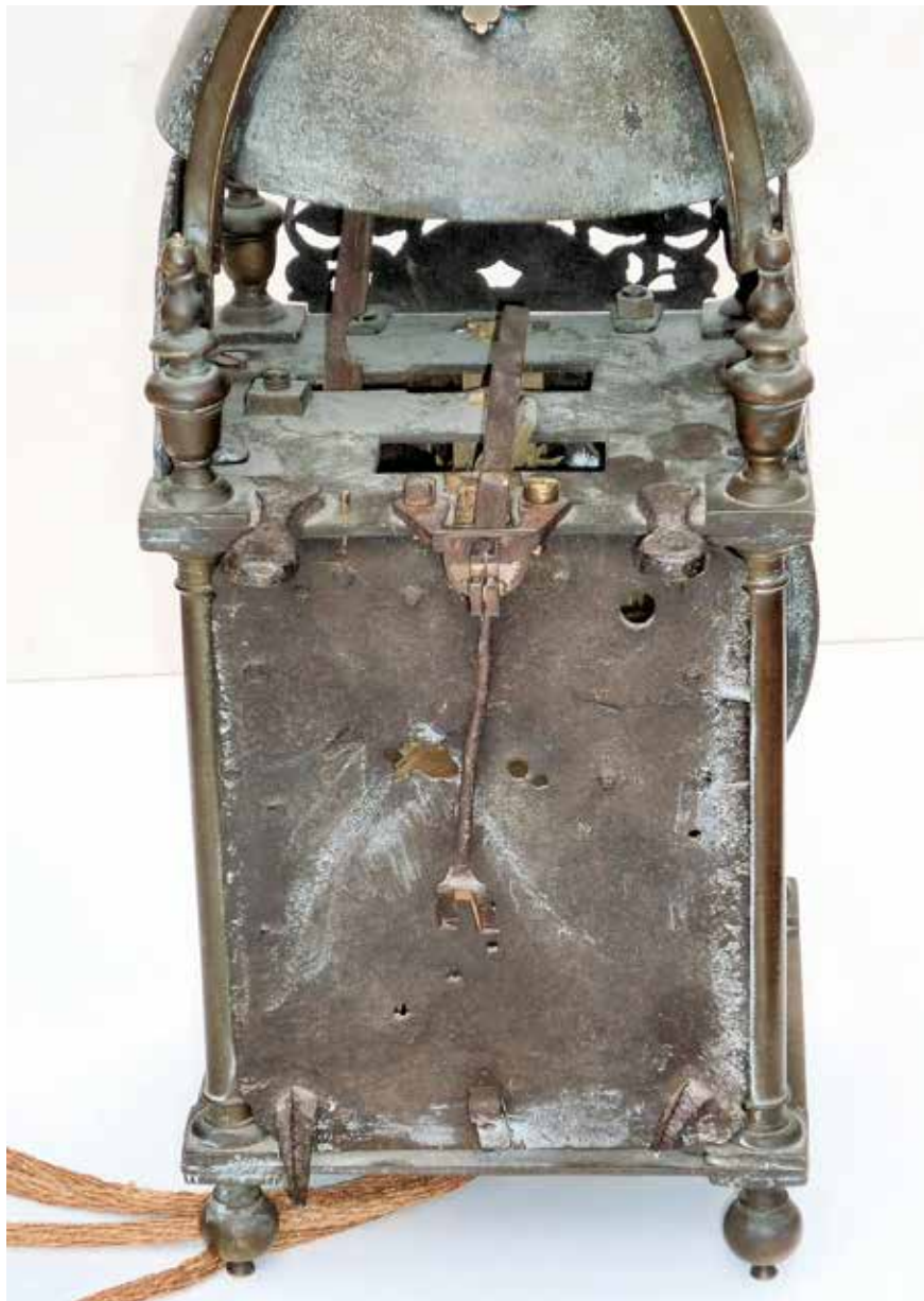
Figure 9. The original iron back plate still carries the spurs. Empty holes show where it once held the original alarmwork and its detent. A small hole by the edge in the centre of the plate is where the detent fitted after the alarm was moved to the left side of the clock.
