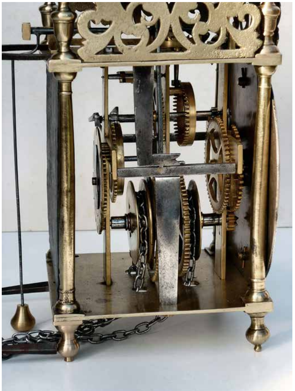
Figure 9. View of the movement of the John Lee lantern clock showing the original verge escapement. Hammer stop end still shaped but in simplified form.
