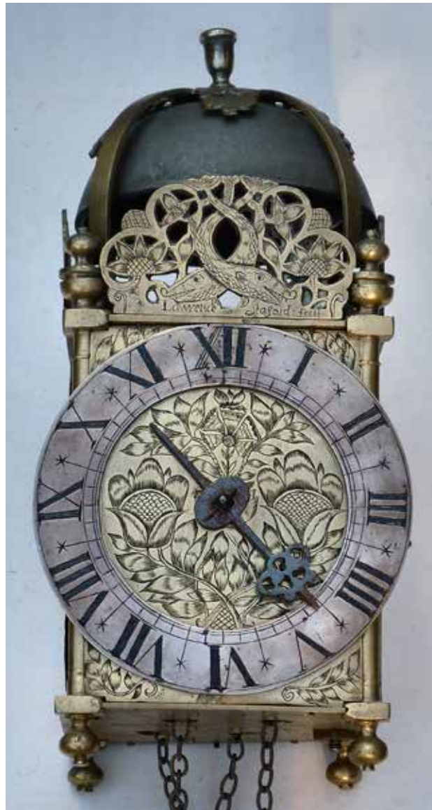
Figure 1. Lantern clock by Lawrence Stafford dating from the 1650s, the oldest Leicester clock so far discovered and by a previously unrecorded clockmaker. Made with balance control, modified later to long pendulum. Very much a provincial clock in style.
