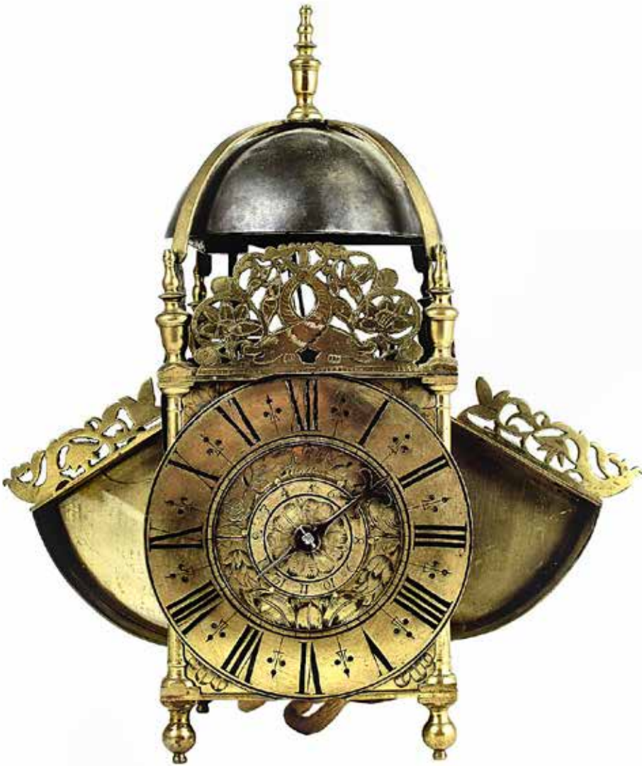
Figure 2 (above). Winged lantern clock with centre swinging verge pendulum and alarmwork made about 1680 by John Wilkins of Leicester. Strong London influence is obvious. Photograph courtesy of Messrs Woolley and Wallis, auctioneers, Salisbury.
