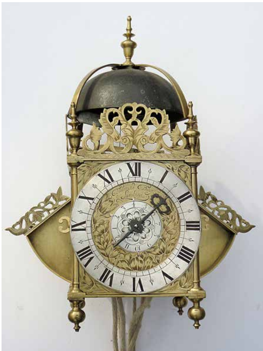
Figure 4. This lantern clock by Thomas Bagley is a winged version, having a centre pendulum, which allowed the alarmwork to be positioned at the back, just as in earlier balance-wheel clocks. Early pendulum lantern clocks often had the pendulum positioned centrally.
