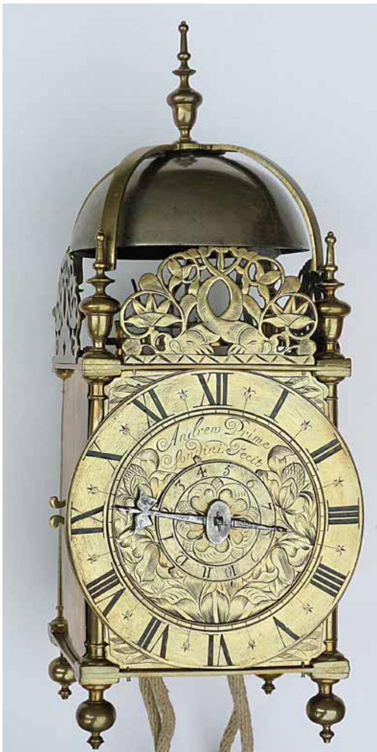
Figure 3. In this lantern clock Andrew Prime uses the specialised frame associated with the Fromanteel family, as also used by Thomas Bagley. The frame is taller, wider and deeper than most.
