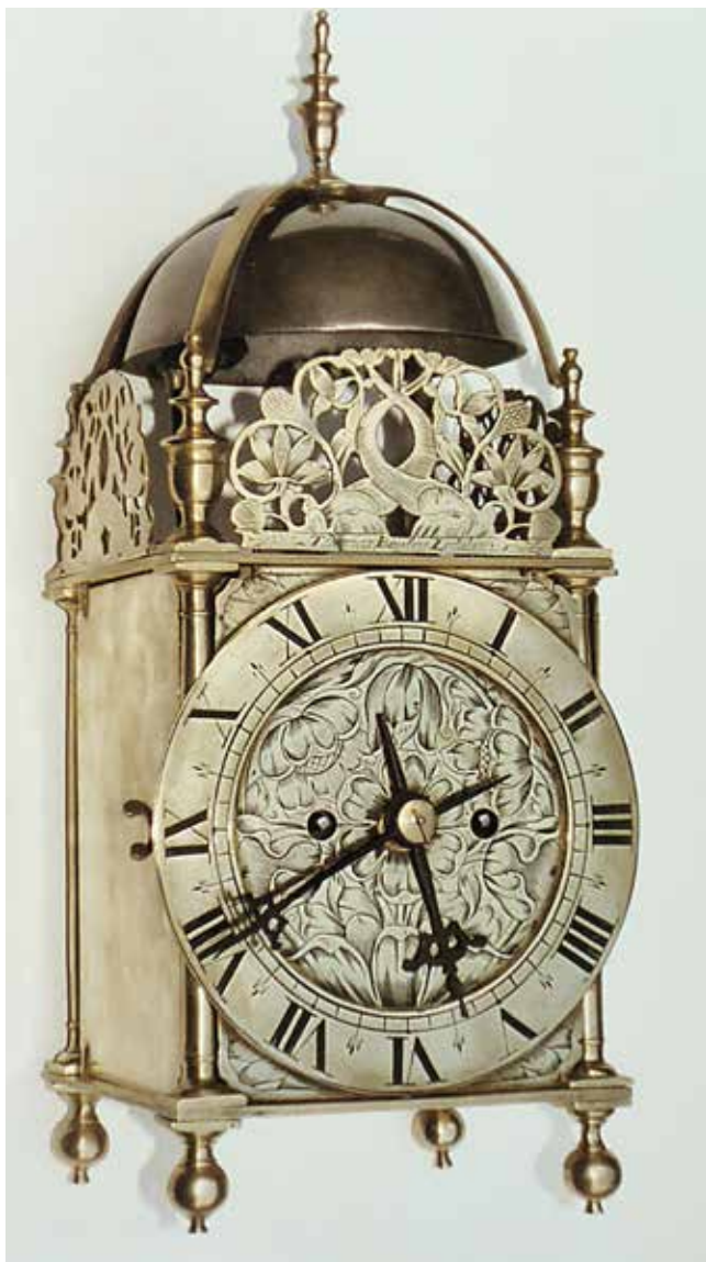
Figure 2. This lantern clock by Thomas Bagley also uses the conventional frame of the day, as used by Thomas Loomes and others. It was probably one of his earlier clocks. It was converted later to a fusee movement.
