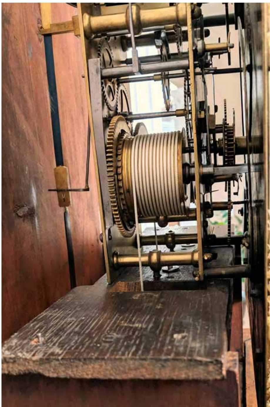
Figure 8. This left view of the movement shows the original seatboard, which is over-wide for this case, which it was clearly not built for. It is also too shallow front to back, whereas an original board would reach far enough to touch the backboard.
