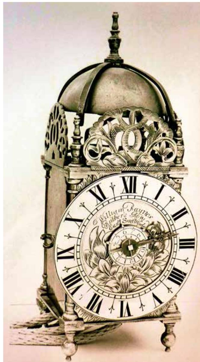
Figure 6. This miniature lantern clock by William Raynes of London is in fact an alarm timepiece, ie non-striking.
