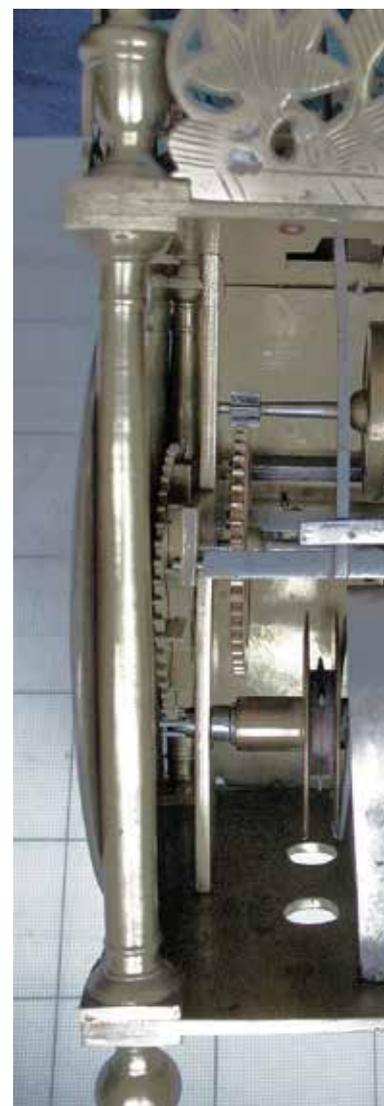
Figure 3. The same clock from the right showing the restored balance wheel escapement. Limited decoration to the hammer stop. Strike fly in line with the wheelwork. Photograph courtesy of Jack and Ann Mcbroom.
