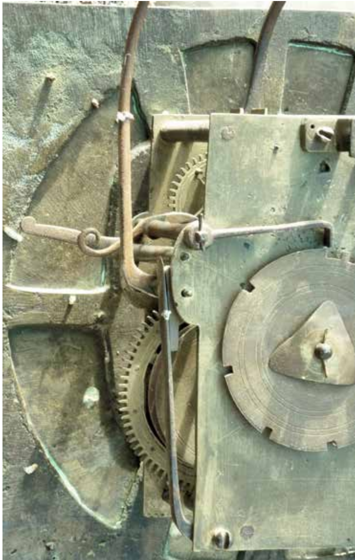
Figure 4. The countwheel trigger close up.
